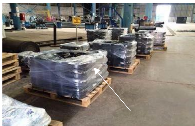
Several wraps of film ensure firmness and stability of the material.
