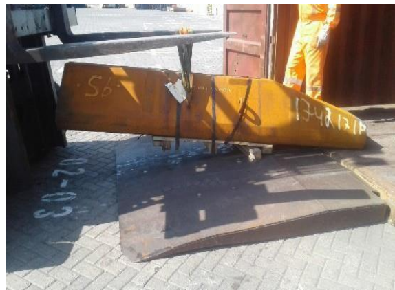
Import lining with insufficient pallet to withstand weight of the material
