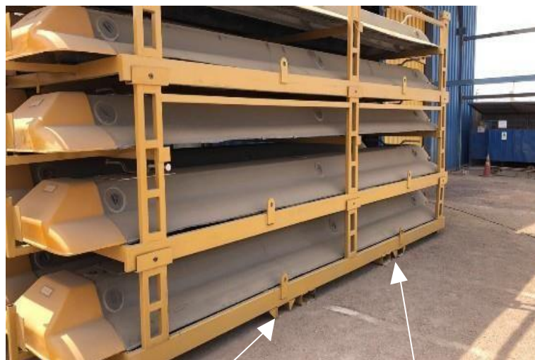
Lectern with shims for Forklift Crane (correct)
