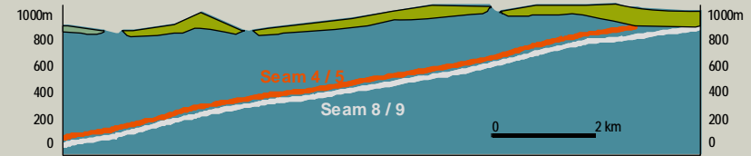
Simple Cross Section – Liulin Coalfield
